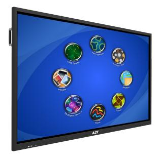
The latest W-series touchscreen now offers an inbuilt Android operating system with up to full 20 touch control. The OPS slot is standard on all models making the integration of attaching the optional slim line PC an easy installation.
